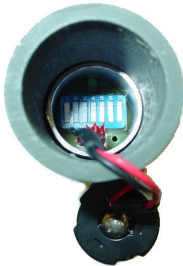
Figure 3: Digital PIR Sensor DIP Switch & LED
