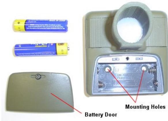
To mount the Wireless PIR motion sensor first remove the battery door and remove the AAA batteries. You will see 2 screw holes in which you can mount a small mounting plate or screw it to the surface of the mounting area.
