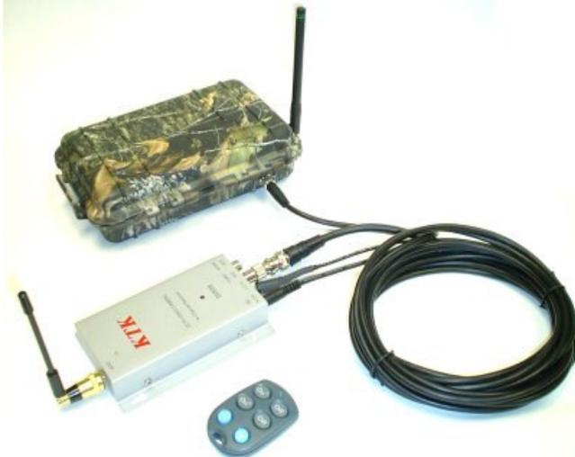
**Recording Setup: Video receiver connected to the Trekker LANC video input with manual KeyFob trigger**
