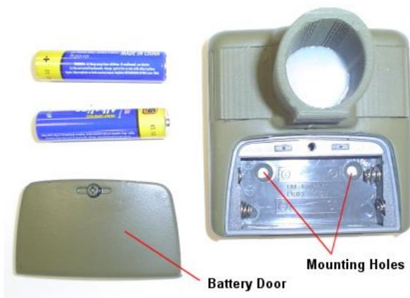
To mount the Wireless PIR motion sensor first remove the battery door and remove the AAA batteries. You will see 2 screw holes in which you can mount a small mounting plate or screw it to the surface of the mounting area.
