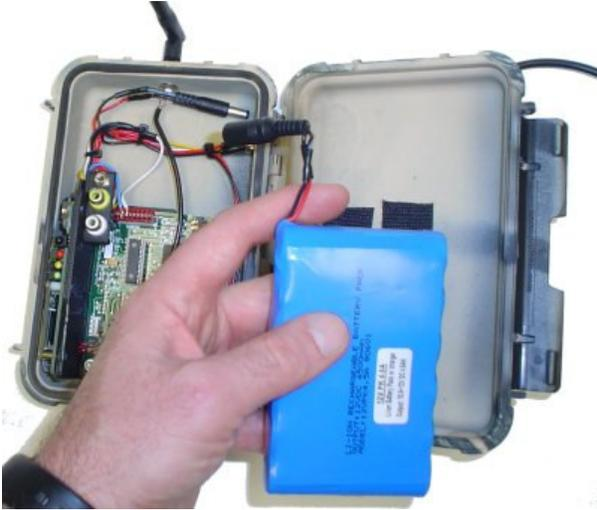
Included with your UndercoverEye unit is a rechargeable 12V Li-Ion battery and 12V charger. The 12V battery is completely removable from the UndercoverEye unit for replacing or recharging. To recharge the 12V battery simply connect the barrel connector to the 12V wall charger unit.
