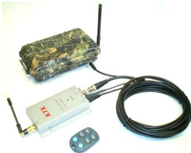
Recording Setup: Video receiver connected to the Trekker MiniDVR video input with manual KeyFob trigger
