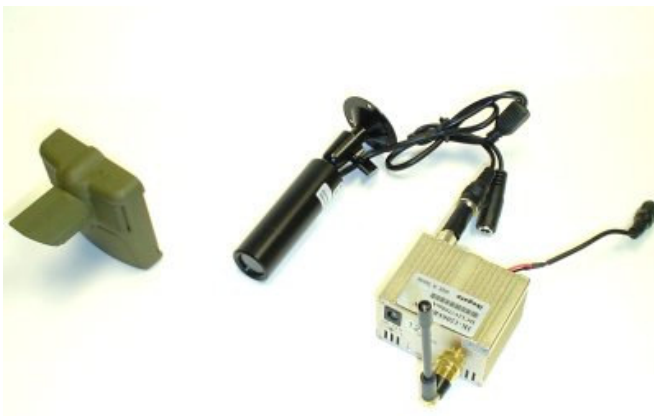
Room setup: PIR Motion sensor trigger, video camera connected to a wireless transmitter
