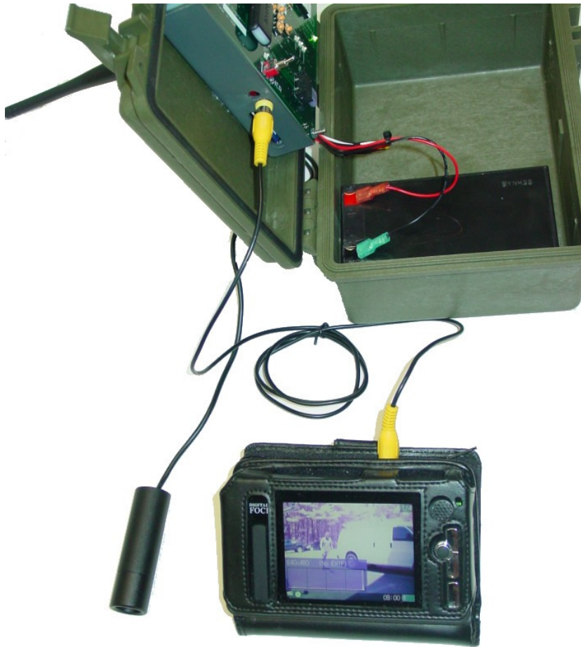
Connecting a TV to view camera during field setup
