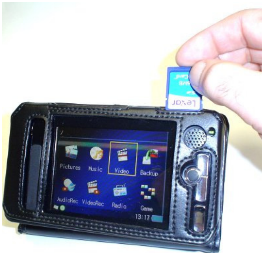
Insert SD Card into PVP
