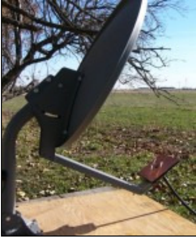
WiFi biquad dish antenna by Eliot Phillips
